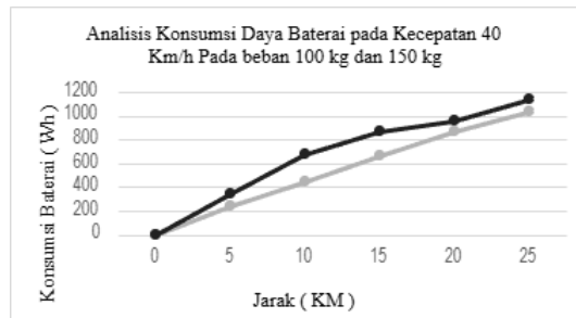
Figure 10. Battery Consumption Test at 40 km/h
