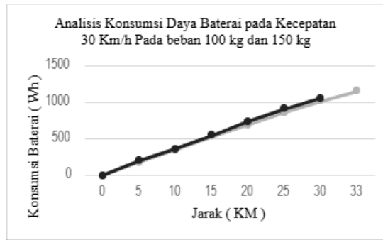
Figure 9. Battery Consumption Test at 30 km/h
