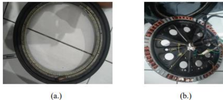
Figure 3. DC wheel-hub motor construction on (a.) rotor and (b.) stator
