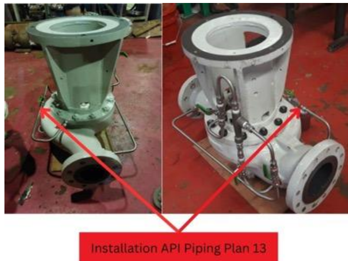
Figure 5. Installation API 682 Piping Plan 13
