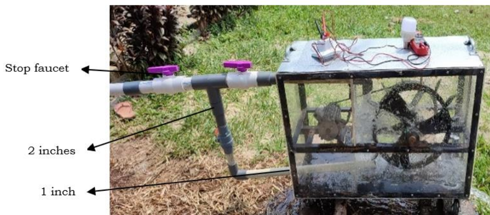
Figure 6. Penstock (PVC Pipe)
